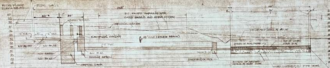
(PROFILE LOOKING SOUTH) SEWAGE DISPOSAL SYSTEM PROFILE SCALE HORIZONTAL 1"=20' VERTICAL 1"=4'
